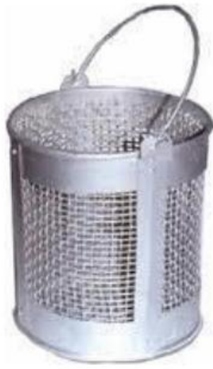
Figure: specific gravity fine aggregate by wire basket (apparatus).
