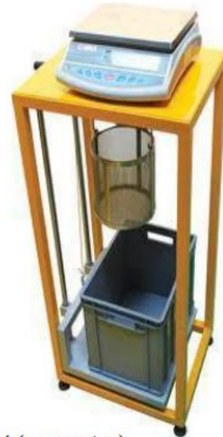
Figure: specific gravity fine aggregate by wire basket (apparatus).
